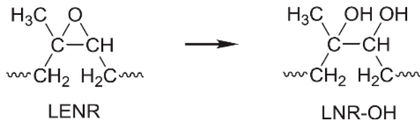
Figure 12. Schematic diagram representing reaction of ELNR to LNR-OH [86].
