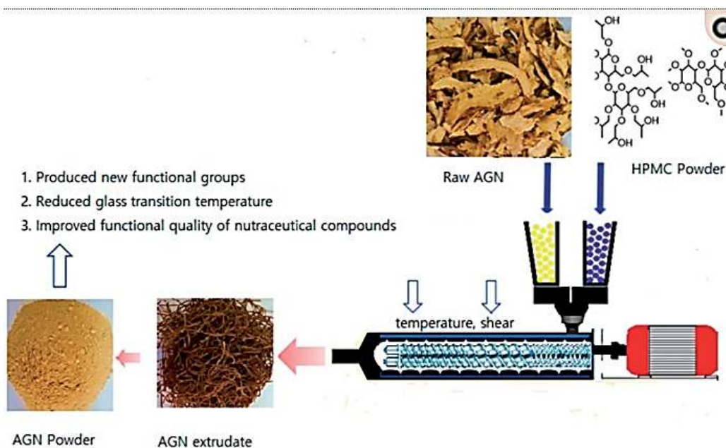
Figure 3. A schematic diagram of the hot melt extrusion process used in the encapsulation of Angelica gigas Nakai (AGN) [38].
