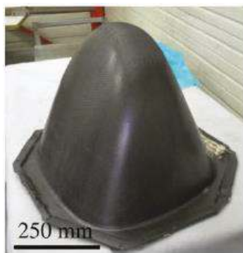
Figure 1. The canopy described in Reference [4] (1:3 scale prototype of the real part).
