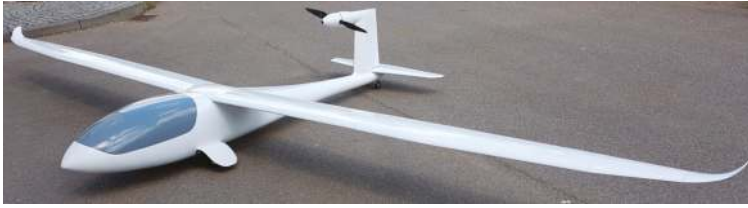
Figure 2. e-Genius-Mod 33.3% free-flight model.
