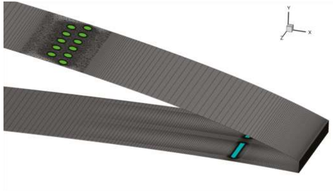
Figure 11. Detail of the CFD surface grid around trailing edge of the AR2 airfoil. The cyan surface represents blowing slots, the green color marks the circular suction holes.
