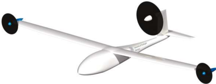
Figure 12. e-Genius-Mod with integrated wing tip propulsion system.
