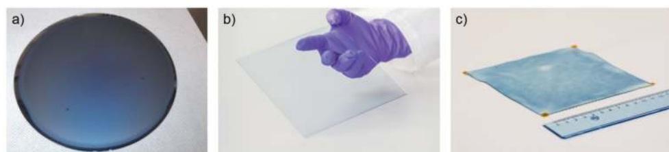
Figure 3. Examples of substrates treated via PRAP-CVD to obtain PEDOT films: (a) silicon wafer (20 cm in dia), (b) glass (15 × 15 cm 2 ), and (c) PET fabric (12 × 12 cm 2 ) [41, 44].
