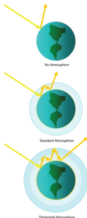
Figure 3.9: Earth Atmosphere Cartoon A cartoon of the greenhouse effect. (Top) Visible light radiation emitted by the sun (yellow arrows) strikes the Earth and reflects as infrared radiation (orange arrow); (middle) an atmosphere reflects some of the infrared radiation back toward the planet; (bottom) a thickened atmosphere reflects greater amounts of infrared radiation. Source: Jonathan H. Tomkin. 12
