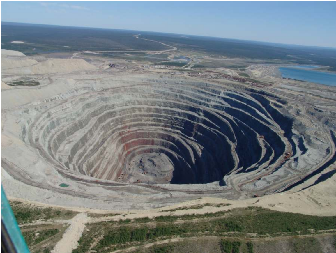
Figure 5.51: A Diamond Mine Udachnaya Pipe, an open-pit diamond mine in Russia, is more than 600 meters (1,970 ft) deep, making it the third deepest open-pit mine in the world. Source: Stapanov Alexander via Wikimedia Commons 70
