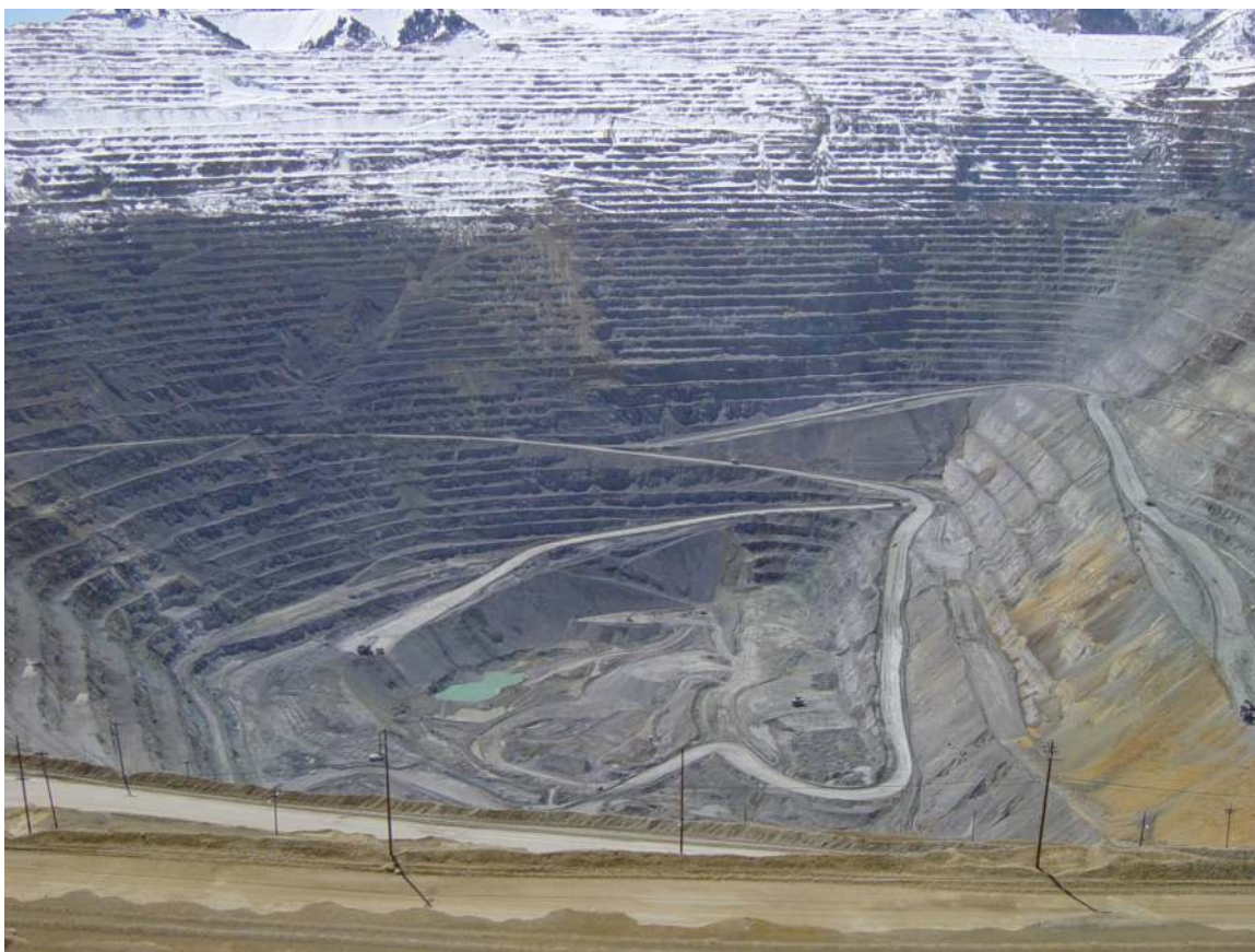
Figure 5.53: Open Pit Mine Bingham Canyon copper mine in Utah, USA. At 4 km wide and 1.2 km deep, it is the world's deepest open-pit mine. It began operations in 1906. Source: Tim Jarrett via Wikimedia Commons 72
