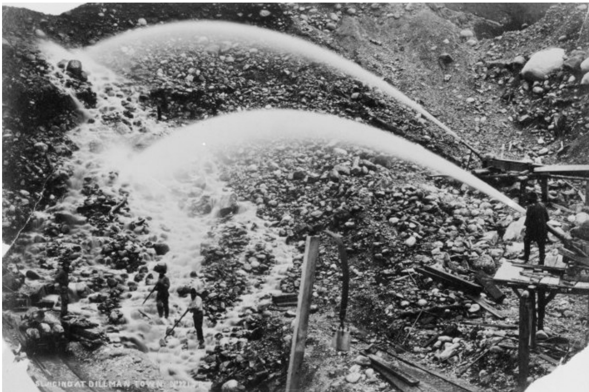
Figure 5.58: Hydraulic Mining Gold hydraulic mining in New Zealand, 1880s Source: James Ring via Wikimedia Commons 79
