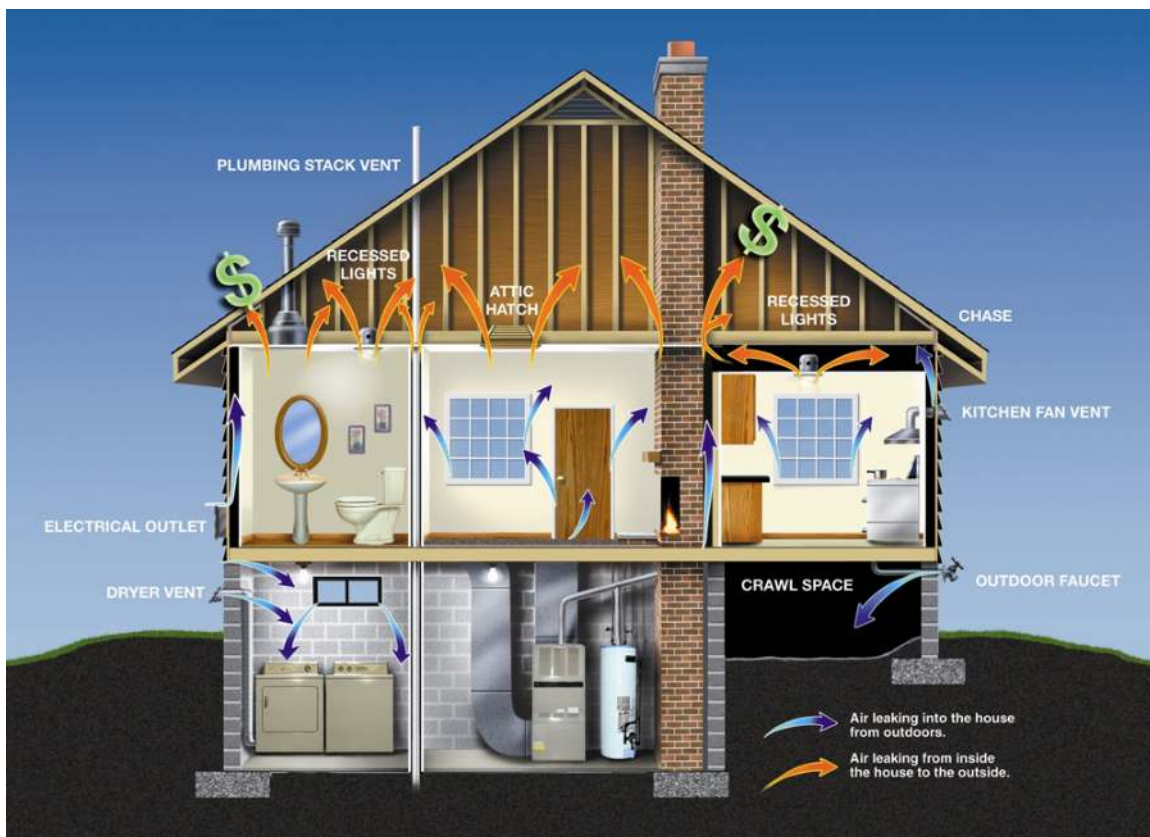
Figure 11.23: Diagram of a Leaky Home Diagram shows the various points in a home where energy may leak. Source: ENERGY STAR 82
