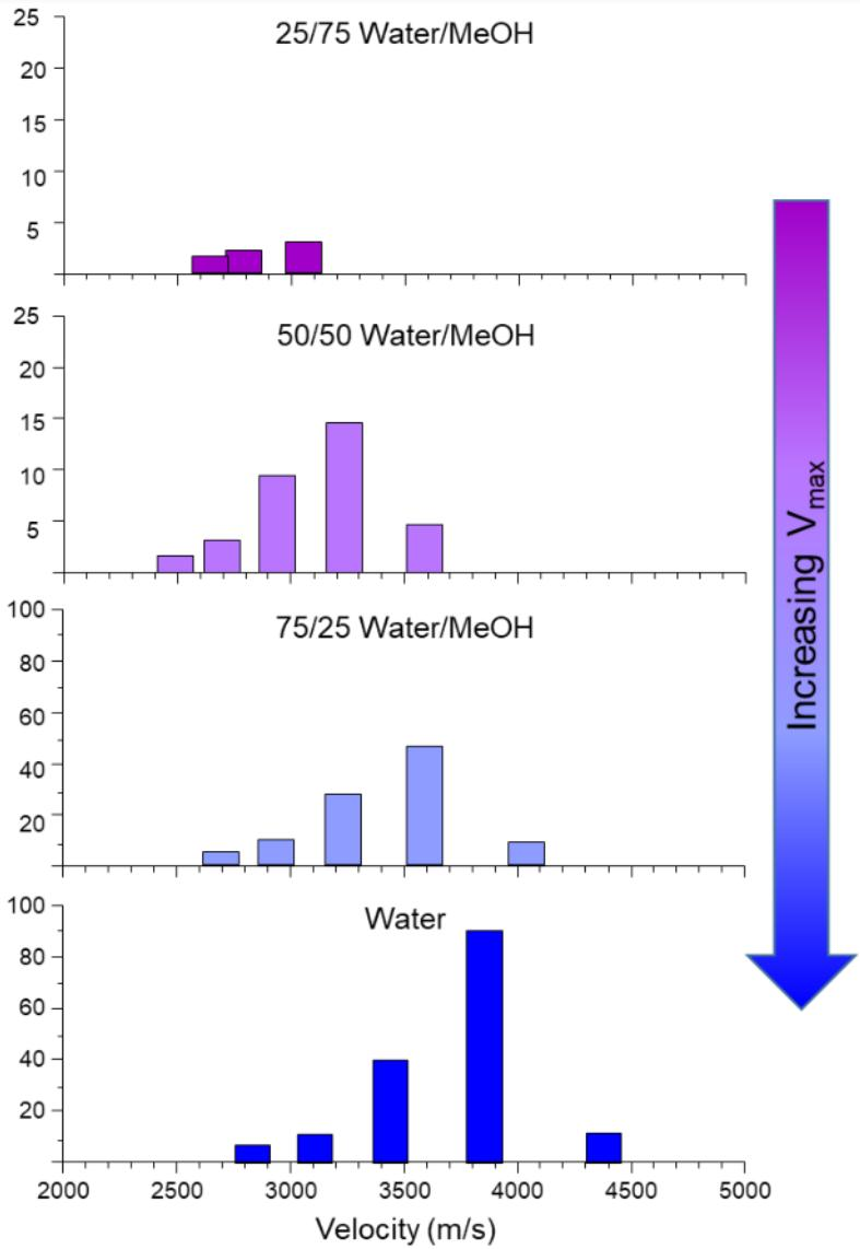
The solvent does impact the LID velocity distribution!
