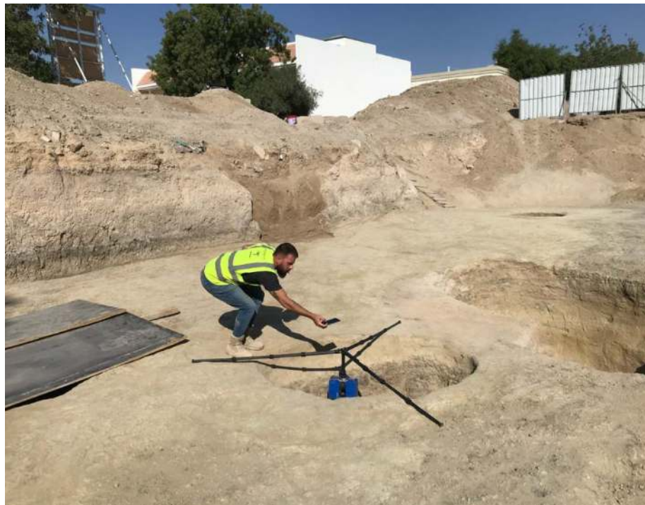
Figure 4: 3-D laser scanning in progress. Recording at all the sites involves production of a 3-D model using either digital photogrammetry or (as here) full 3-D laser scanning.
