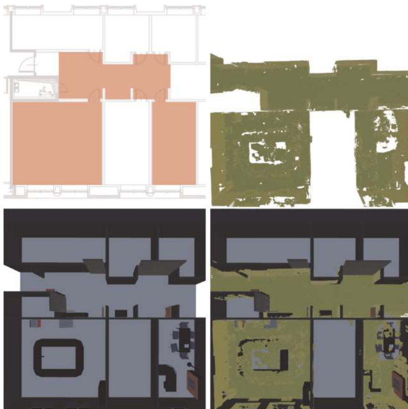
Figure 6. Top-left image: the map used to model the virtual environment. The red zone indicates the game area. Top-right image: the scanned map obtained using the SLAM feature of the HoloLens. Bottom-left image: the virtual environment. Bottom-right image: notice the matching of the virtual environment with the scanned map.
