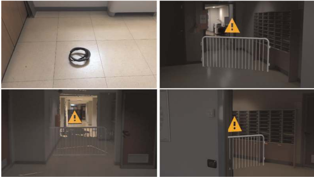
Figure 7. Top-left image: the pre-defined starting position of the HoloLens. Top-right image: an example of virtual barrier employed to limit the ARP's movements. Bottom-left image: in the background it is possible to visualize the contrast between the real environment and the black material used to make invisible the scanned environment. Bottom-right image: an example of occlusion between a real (the door) and a virtual object (the barrier).
