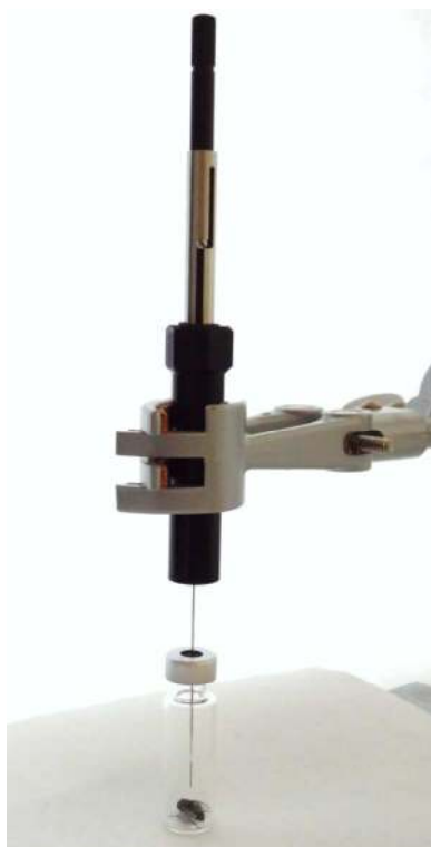
Fig. 2. Static headspace sampling of insect volatiles with a SPME device.
