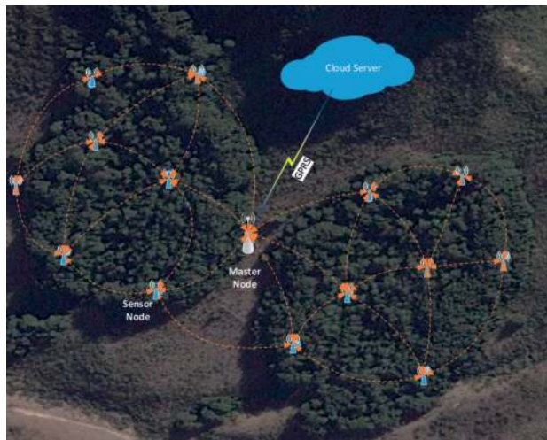
Figure 8. WSN mesh network architecture.
