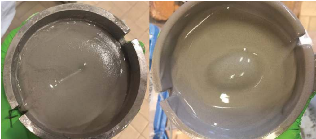
Figure 6.14 Image of the bottom plate after the test with variation in flow area and without magnetic field (left) A_1 – agglomeration of particles leading to blocking; (right) A_2 – no agglomeration of particles at the slit resulting in full flow. Source: [39].
