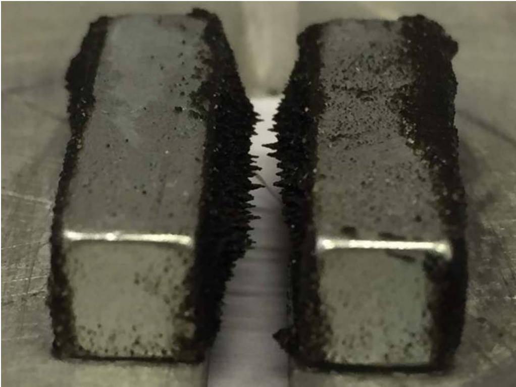
Figure 6.11 Deposition of magnetizable particles as visible after gently rinsing off the paste from the bottom plate (Courtesy C. Chibulu).
