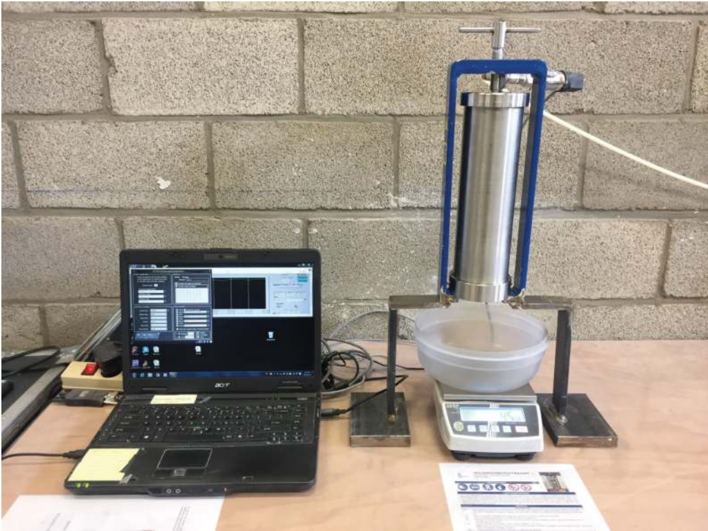
Figure 6.5 A photograph showing the experiment set-up for the study of leakage (Courtesy C. Chibulu).
