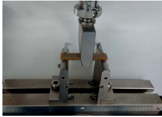
Figure 2. Assembly used for flexural test (according to ASTM D790).
